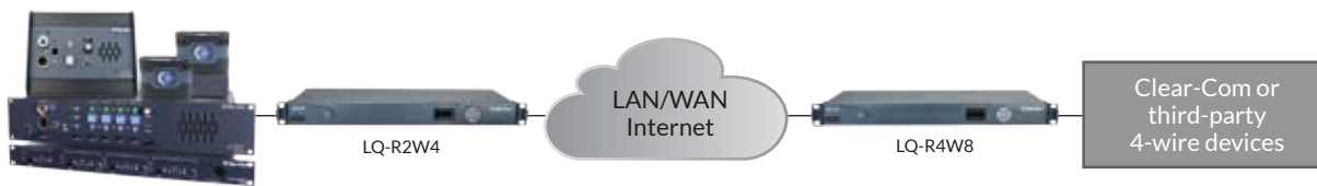
Linking 2-wire with 4-wire intercom system
