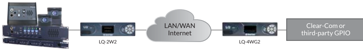
Linking 2-wire intercom system to GPIO
