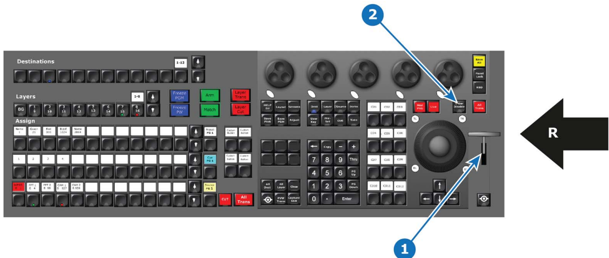
Image 10-11 1 T-Bar 2 T-Bar disable button R Right Side of the Controller
