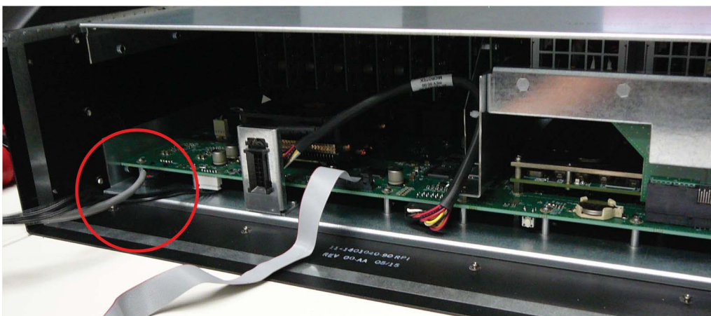
Image 14-35 USB Ext Cable connected to the Motherboard
