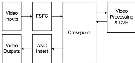
Figure 6: Video Flow Through the Switcher
