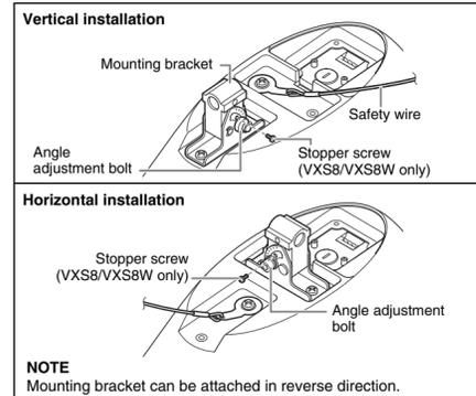
2 Set the desired vertical angle of the speaker. Loosen the angle adjustment bolt with the supplied hexagon wrench, adjust the angle of the speaker, and tighten the angle adjustment bolt to fix the speaker (indication of torque: 8 N·m).
